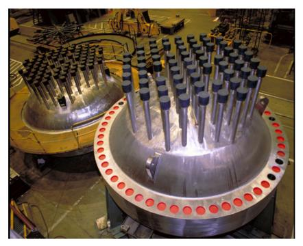
In the EPR there are 89 potential CRDM severances with severe LOCA potential. Whether the Alloy 690 in service will prove more sustainable and resistant to stress corrosion cracking than the Alloy 600 in the coming 60 years of operation is yet to be known.
